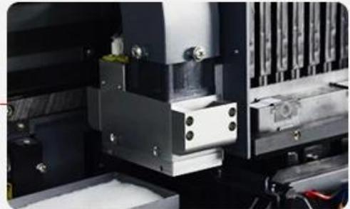
② Damper is the part to connect print head with ink supply and stock the ink temporarily for printer head. Damper must be kept sealed when machine is working.
