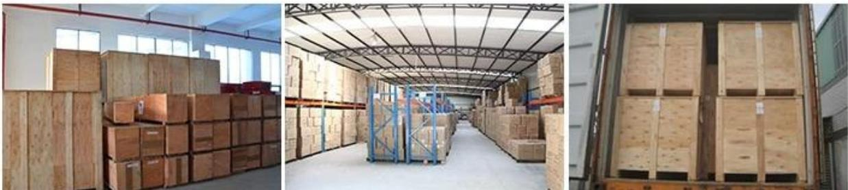
Before shipment, the machine is cleaned fully, daubed by anti-rust oil carefully, covered by plastic bag, wrapped by the stretch film, and at last firmed into the wooden case.
