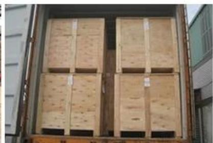
Before shipment, the machine is cleaned fully, daubed by anti-rust oil carefully, covered by plastic bag, wrapped by the stretch film, and at last firmed into the wooden case.
