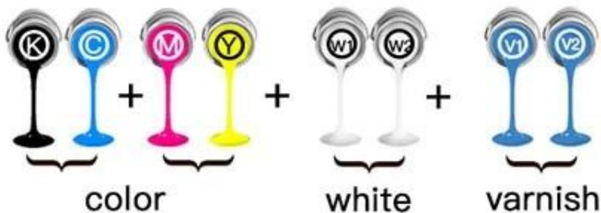
**EPSON DX5 Print Heads Arrangement (1pc Head)**
