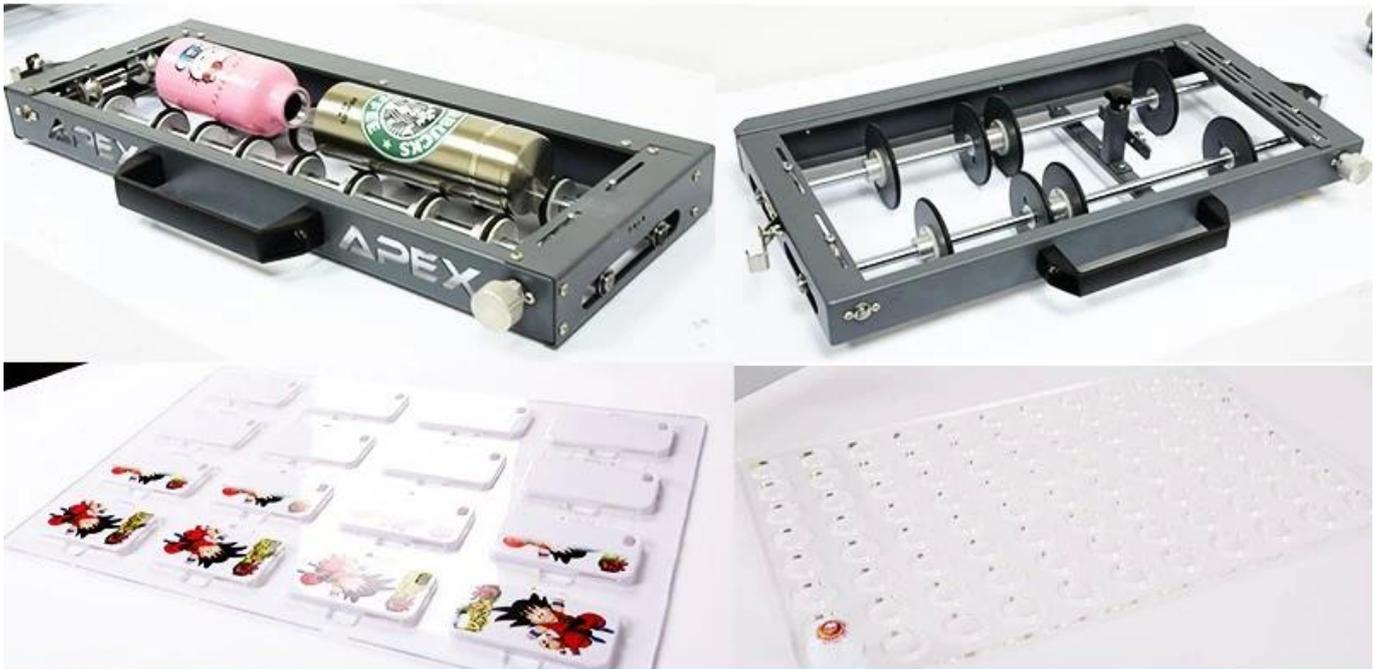
To increase the output of production for special product, Apex supplies specific fixture which makes it possible to implement a batch printing. Contact Now, to custom your unique fixtures for special items.
