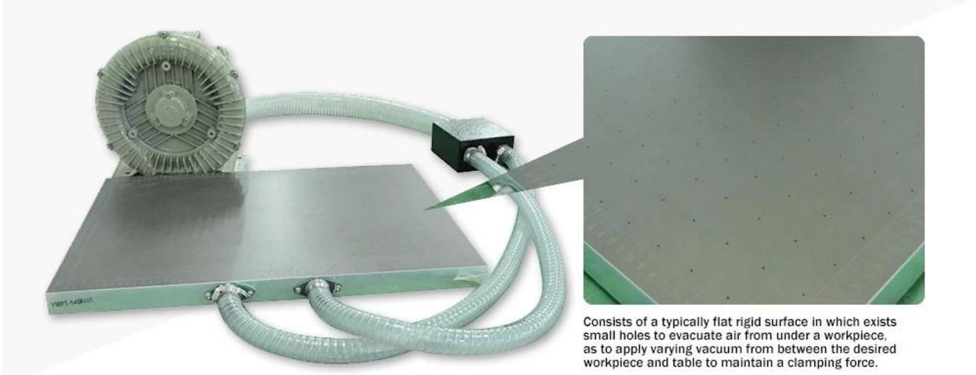
Consists of a typically flat rigid surface in which exists small holes to evacuate air from under a workpiece, as to apply varying vacuum from between the desired workpiece and table to maintain a clamping force.
