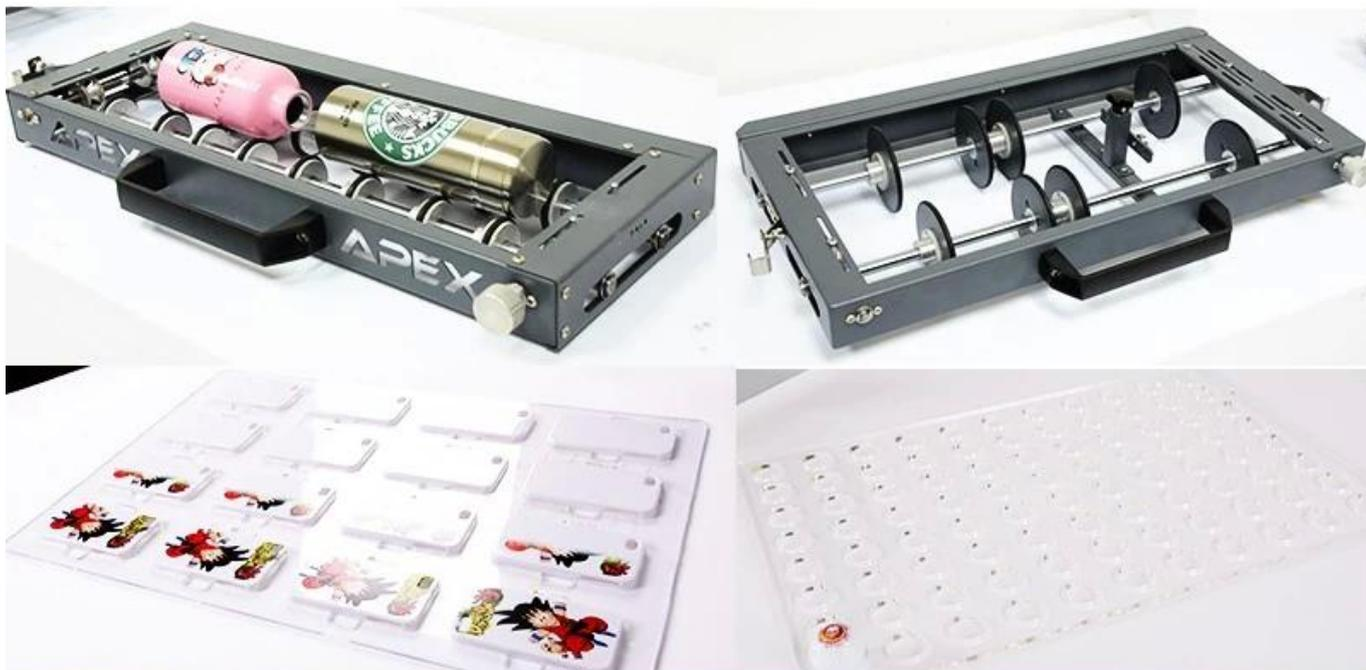
To increase the output of production for special product, Apex suplys specific fixture which makes it possible to implement a batch printing. Contact Now, to custom your unique fixtures for special items.
