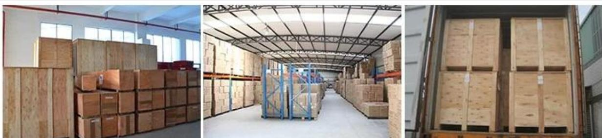
Before shipment, the machine is cleaned fully, daubed by anti-rust oil carefully, covered by plastic bag, wrapped by the stretch film, and at last firmed into the wooden case.
