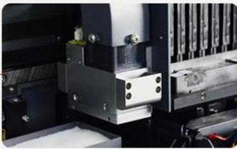
**2** Damper is the part to connect print head with ink supply and stock the ink temporarily for printer head. Damper must be kept sealed when machine is working.
