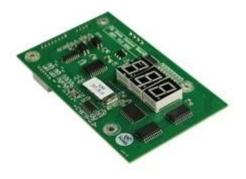
This lifting board is used to control motor up and down
