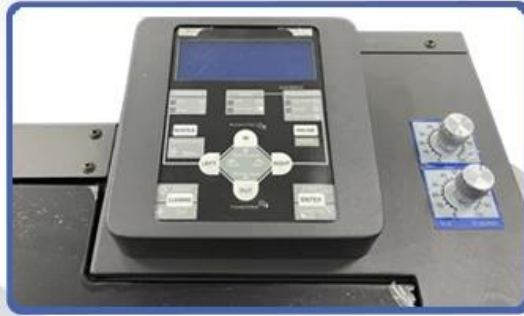
NO.2 Digital Operation Display System
