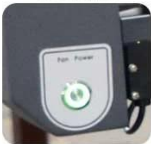
Additional Fan to Absorb the Flying Ink
