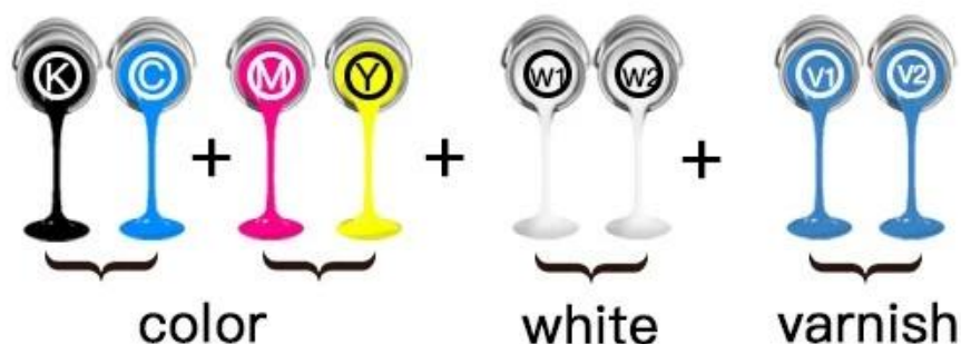
EPSON DX5 Print Heads Arrangement (1pc Head) UV4060/UV6090/N4060/N6090: Single Head 8 Channels
