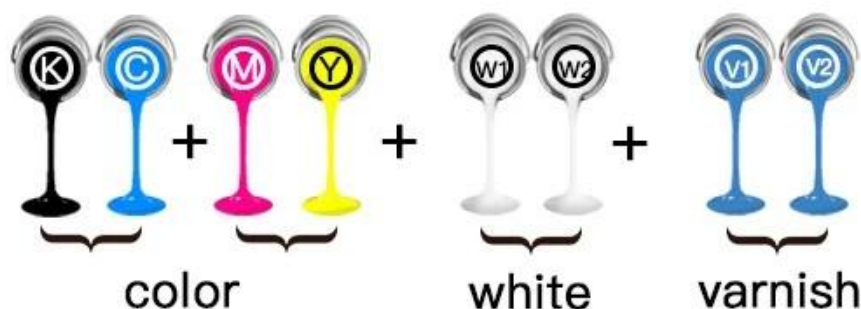
EPSON DX5 Print Heads Arrangement (1pc Head) UV4060/UV6090/N4060/N6090: Single Head 8 Channels
