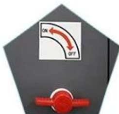
Suction platform segment control
