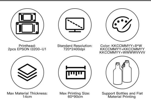
Equipped with double I3200-U1 print heads, color mode KKCCMMYY+ 8\*W / KKCCMMYY+KKCCMMYY/KKCCMMYY+WWWWVVVV, you can get faster printing speed and enhance productivity.
