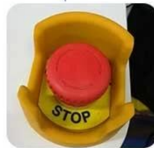
Emergency Stop Button
