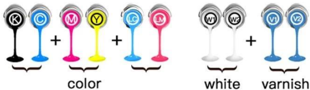
Toshiba CE4 Print Heads Arrangement (5~12pcs Heads Options) UV1610GM: Single Head Single Color
