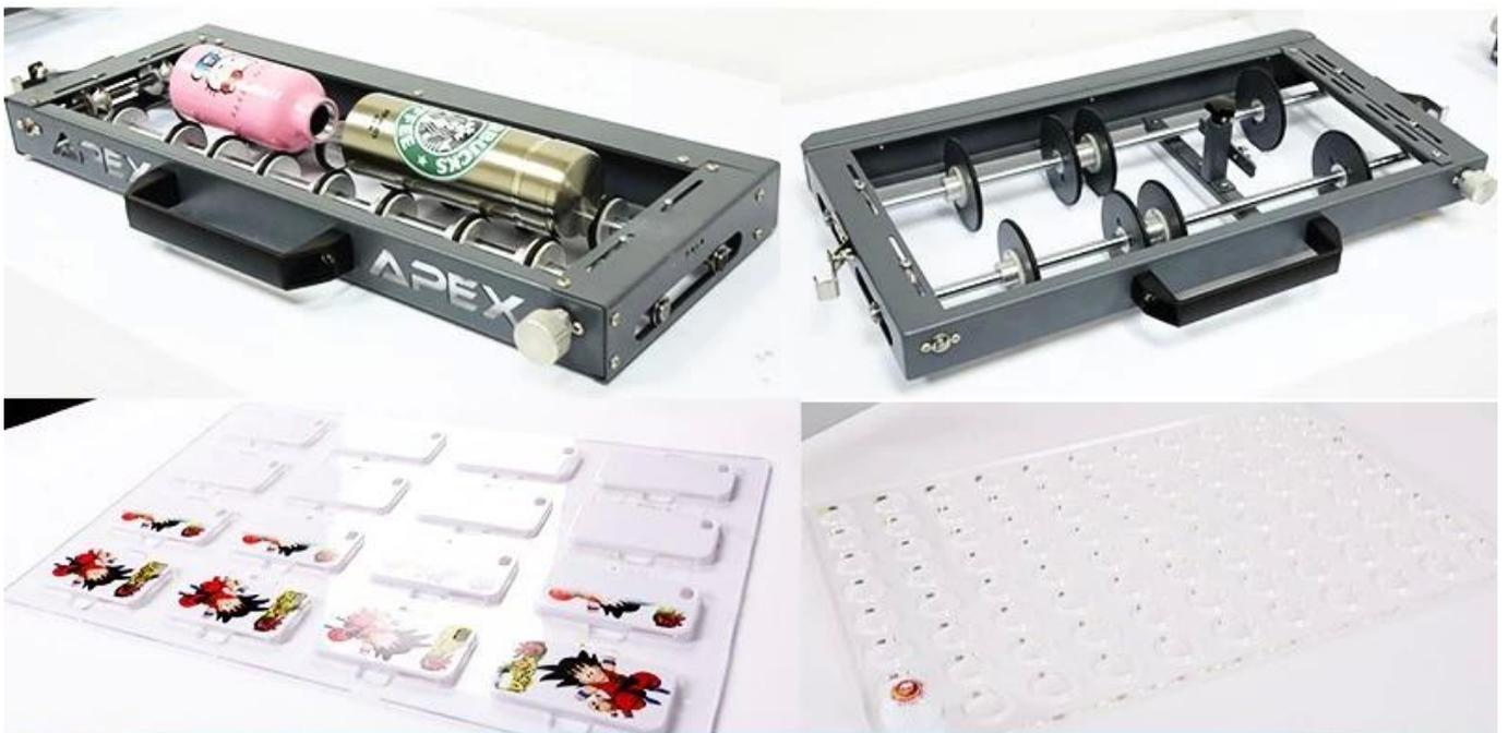
To increase the output of production for special product, Apex supplies specific fixture which makes it possible to implement a batch printing. Contact Now, to custom your unique fixtures for special items.
