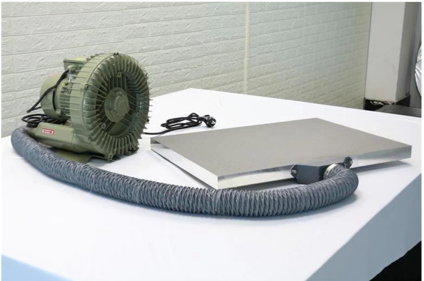
Consists of a typically flat rigid surface in which exists small holes to evacuate air from under a workpiece, as to apply varying vacuum from between the desired workpiece and table to maintain a clamping force.
