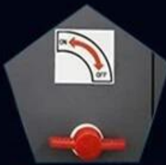
Suction platform segment control
